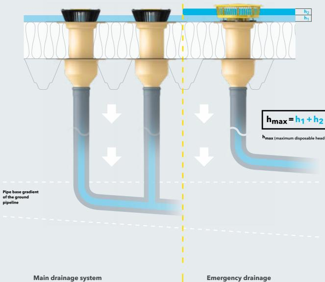
The principle of conventional drainage: The water drains through multiple fall pipes into a ground pipe with a gradient and gets discharged then via this pipe. However, in case of heavy rainfall incidents the main drainage system reaches its capacity limits. This is where the emergency drainage system kicks in - from a precisely defined head of water.
