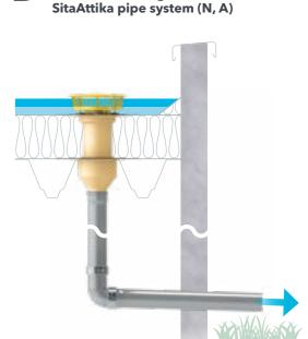
SitaStandard, vertical, with extension unit and retaining element with
